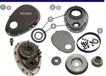
Belt drive kits help to restore power loss caused by original timing gear wear and stretching. Helps reduce noises associated with valve train and dampens out certain harmonic noises generated by the three main bearing 'A' series engine. Also preserves exact timing where anything over 2° out causes power loss. The kits available contains everything to replace timing gears and cover. Mini Spares latest belt drive kits which have a plastic dust cover will
